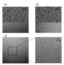
Fig. 14 Cryo-TEM images obtained for 2 wt% solutions. (a) PamCSK, (b)  $Pam_2CSK4$ , (c)  $Pam_3CSK4$ . Enlarged images are shown at top in (a) and (b) and to the right in (c). <sup>71</sup>
