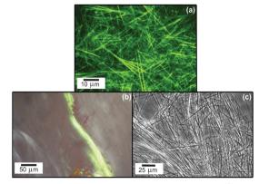
Fig. 16 Fibrillar superstructure of peptide amphiphile Matrixyl. 72 (a) Confocal optical microscopy image (fluorescent labelling with rhodamine B, 0.014 wt% Matrixyl in water), (b) apple green birefringence observed by polarized optical microscopy upon staining with Congo red, (c) differential optical microscopy image (1 mg ml $^{-1}$  = 0.1 wt%).
