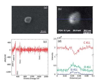
Fig. 6 (a) In-Lens SEM image of a  $\cong 30$  nm silica nanoparticle deposited on a carbon foil of a TEM grid, (b) SEM image of the same particle acquired in the SAM instrument, (c) AES point spectrum taken on the center of the particle identified in (b) and (d) AES line scans across the particle. The line scan position is displayed in (b) with a blue line
