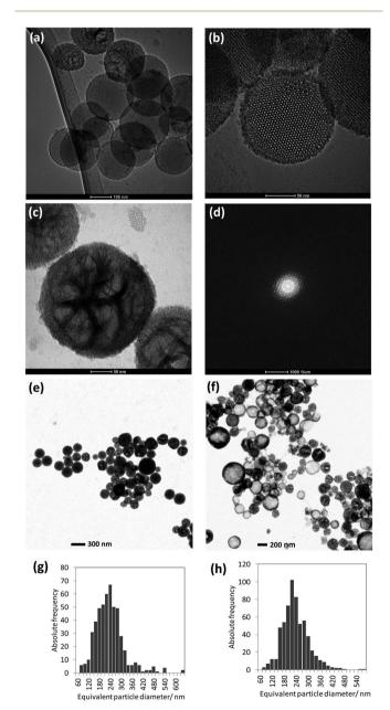
Fig. 2 (a-c) TEM images of silica NNV-001 particles, (d) diffraction pattern obtained from the particle displayed in (b), (e) T-SEM image of the as-prepared dispersion, (f) T-SEM image of the aged dispersion, (g) histogram showing the particle size distribution of the freshly prepared dispersion as measured by T-SEM and (h) histogram with the particle size distribution of the aged dispersion as measured by T-SEM.
