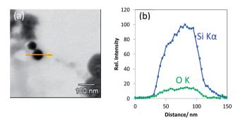
Fig. 5 (a) T-SEM image of a silica nanoparticle ( $d \approx 65$  nm) with an arrow indicating the EDX line scan position and (b) EDX line scan with Si K $\alpha$  signal and O K $\alpha$  signal of the particle shown in (a).
