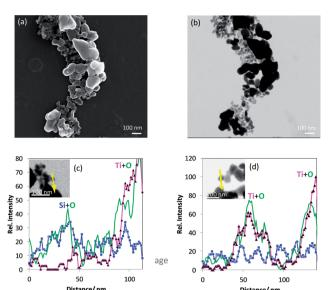
Fig. 12 (a) In-Lens SEM and (b) T-SEM image of nominal silane coated titania nanoparticles, (c and d) EDX line scans of elements Si (blue squares), O (green line, no symbol) and Ti (magenta triangles) together with T-SEM images (inserts) of a titania-silane aggregated nanomaterial. Yellow arrows represent the EDX line scan positions.
