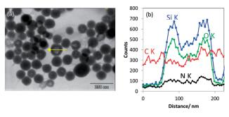
Fig. 10 (a) T-SEM image of non-porous silica nanoparticles modified with IPTES deposited on carbon foil coated copper grid and (b) EDX line scan measured along a particle as indicated by the arrow in (a).
