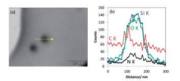
Fig. 9 (a) T-SEM image of non-porous silica nanoparticles covered by an IPTES shell that were deposited on a Substratek $^{\text{TM}}$  grid as a low-carbon substrate for analysis, (b) EDX line scan measured along the particle as indicated by the arrow in (a).
