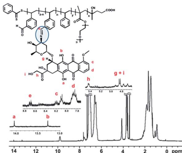
Fig. 3 <sup>1</sup>H NMR spectrum taken after doxorubicin conjugation to the nanoparticles.
