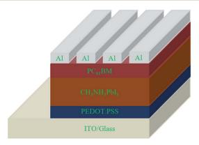
Fig. 1 Structure of CH<sub>3</sub>NH<sub>3</sub>PbI<sub>3</sub>/PC<sub>61</sub>BM solar cells.
