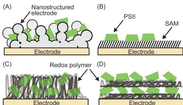
**Fig. 6** Immobilisation strategies for PSII on electrodes. (A) Incorporation of PSII into the nanopores of a nanostructured electrode, (B) immobilisation of PSII via a self-assembled monolayer (SAM), (C) entrapment of PSII in a redox polymer and (D) layer-by-layer (LBL) assembly of PSII and redox polymer.
