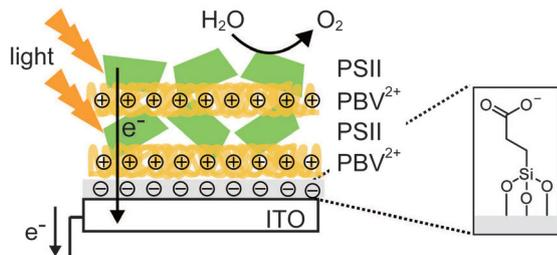
Fig. 9 Layer-by-layer (LbL) assembly of PBV<sup>2+</sup> and PSII on an ITO-coated glass substrate.<sup>33</sup>
