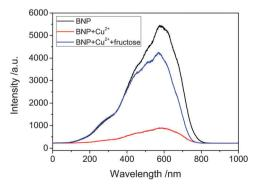
Fig. 4 Emission spectra of BNP (10 mM), BNP plus 5 equiv. Cu<sup>2+</sup> and BNP-Cu<sup>2+</sup> plus 5 equiv. fructose with two-photon excitation at 910 nm.
