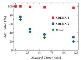
Fig. 2 Changes of the absorbances due to the carbazole dyes (ADEKA-1, ADEKA-2 and MK-2) adsorbed on the  $TiO_2$  electrodes with the soaked time into 3-methoxypropionitrile—water (1:1 in volume) at 85 °C in the dark.
