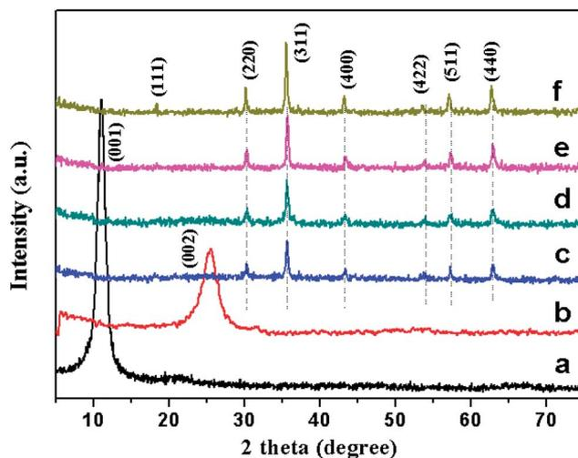
**Fig. 2** XRD patterns of GO (a), RGO (b), RGO-Fe<sub>3</sub>O<sub>4</sub>-1 composite (c), RGO-Fe<sub>3</sub>O<sub>4</sub>-2 composite (d), RGO-Fe<sub>3</sub>O<sub>4</sub>-3 composite (e) and Fe<sub>3</sub>O<sub>4</sub> NPs (f).
