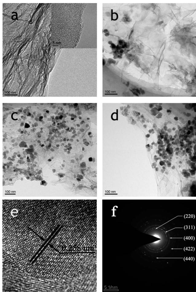
**Fig. 1** TEM images of RGO (a), RGO-Fe<sub>3</sub>O<sub>4</sub>-1 composite (b), RGO-Fe<sub>3</sub>O<sub>4</sub>-2 composite (c), RGO-Fe<sub>3</sub>O<sub>4</sub>-3 composite (d); HRTEM image (e) and SAED pattern (f) of RGO-Fe<sub>3</sub>O<sub>4</sub>-2 composite.
