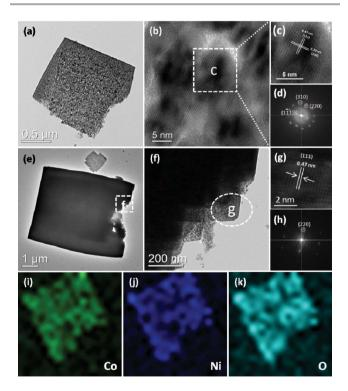
**Fig. 4** (a–d) TEM, HRTEM images and SAED pattern of NiCo $_2$ O $_4$  nanosheets obtained from a hydrothermal reaction time of 3 h; (e–h) TEM, HRTEM images and SAED pattern of NiCo $_2$ O $_4$  hierarchical cubic microstructures consisting of NiCo $_2$ O $_4$  nanosheets obtained from a hydrothermal reaction time of 6 h; and (i–k) The corresponding EDX elemental mapping images of NiCo $_2$ O $_4$  nanosheets obtained from a hydrothermal reaction time of 3 h.
