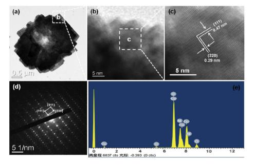
Fig. 5 (a-e) TEM, HRTEM images, SAED pattern and the EDS spectrum of NiCo<sub>2</sub>O<sub>4</sub> hierarchical flower-like super-structures consisting of porous NiCo<sub>2</sub>O<sub>4</sub> nanosheets.
