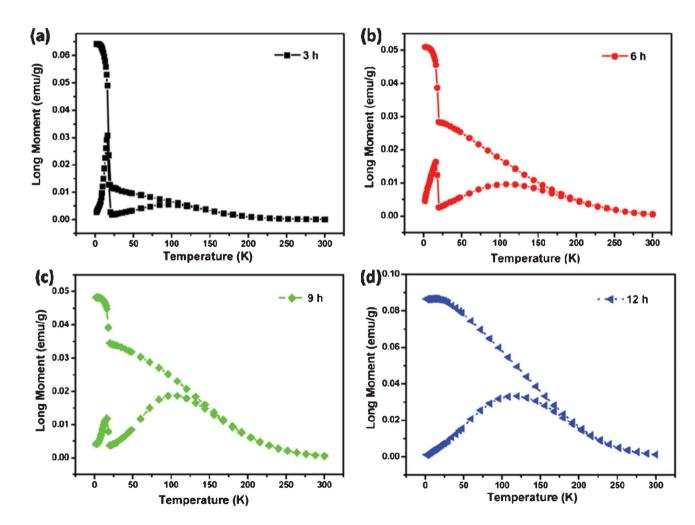
Fig. 9 (a-d) ZFC-FC curves of NiCo<sub>2</sub>O<sub>4</sub> samples at 100 Oe.
