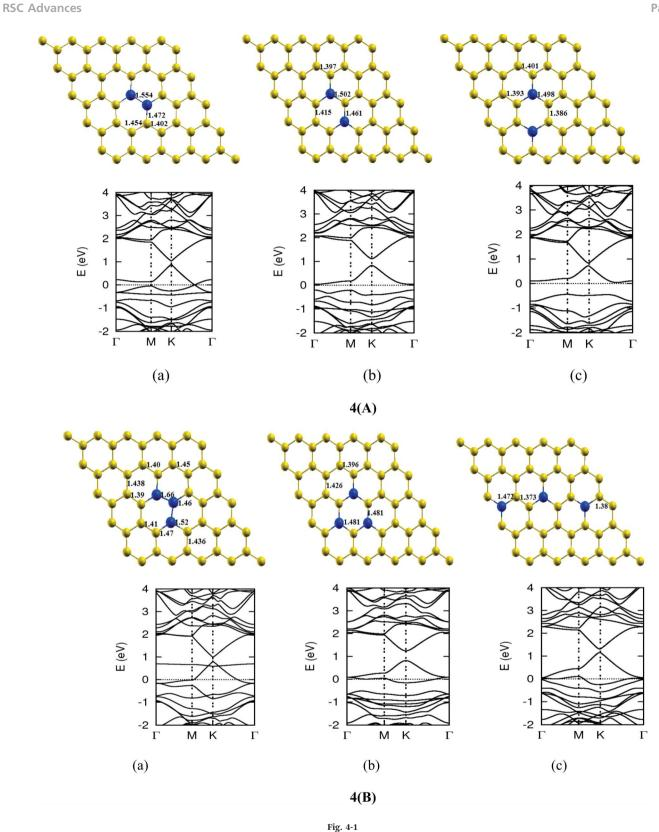
resulting in p-type doping. Another important observation that can be made is regarding breaking of the symmetry of two graphene sublattices because of the introduction of a B atom, now introducing an energy gap of 0.14 eV around the Dirac point. This changes the behavior of graphene from semi-metal to conductor. The charge transfer was also calculated using Bader charge analysis, which shows 1.79 e charge transfer from boron to carbon. The results are in agreement with
