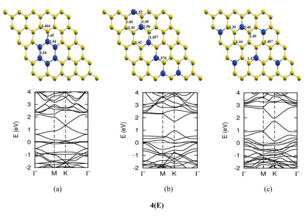
Fig. 4-3 Some optimized geometries and band structures of two, three, four, five and six B atom doped graphene sheet in (A), (B), (C), (D) and (E), respectively. The upper rows in these show geometrical structures and bottom rows present the band structures.
