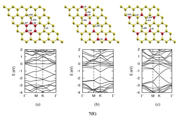
Fig. 7-3 Optimized geometries and band structures of two, three, four, five and six N atom doped graphene sheet in (A), (B), (C), (D) and (E), respectively. The upper rows in these show geometrical structures and bottom rows present the band structures.
