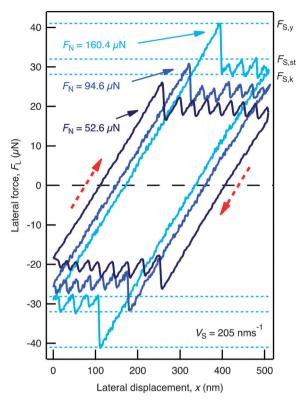
**Fig. 2** Friction loops, showing  $F_1$  as a function of  $x_S$  at a constant film thickness of i = 7 and for three different values of  $F_N$ . The velocity is constant at  $v_S = 205$  nm s<sup>-1</sup>, and the back-and-forth displacement is in the directions indicated by (red) dashed arrows. Friction features  $F_{S,v}$ ,  $F_{S,k}$ , and  $F_{S,st}$  are defined for the  $F_N = 160.4 \,\mu\text{N}$  trace.
