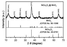
Fig. 1 XRD pattern of hierarchical NiCo<sub>2</sub>O<sub>4</sub>@MnO<sub>2</sub> core-shell heterostructured NW arrays scratched from Ni foam.
