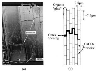
**Fig. 10** (a) Cross-section of abalone shell showing how a crack, starting at the left, is deflected by the viscoplastic layer between calcium carbonate lamellae; (b) schematic drawing showing the arrangement of calcium carbonate in nacre, forming a miniature "brick and mortar" structure. <sup>97</sup>
