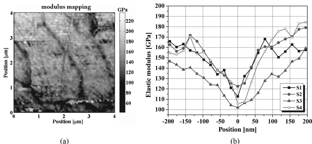
**Fig. 18** (a) Map of elastic modulus taken from the nacre layer at a depth of 300 μm beneath the inner surface of the bivalve shells of *Perna canaliculus*; (b) the modulus change across organic–inorganic interfaces.<sup>110</sup>
