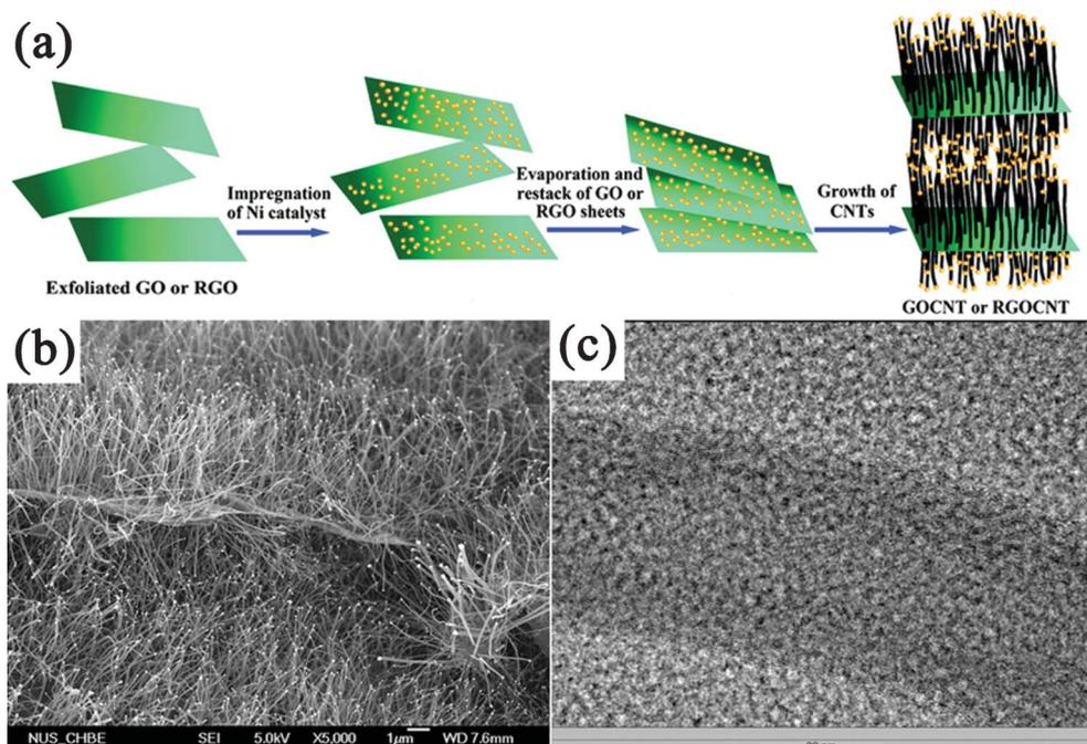
**Fig. 6** (a) Scheme illustrating the experimental steps of pillaring GO/RGO platelets with CNTs. (b) Field emission SEM (FESEM) and (c) TEM images of the CNT-pillared GO nanosheets. Reprinted with permission from ref. 328, Copyright 2010, American Chemical Society.
