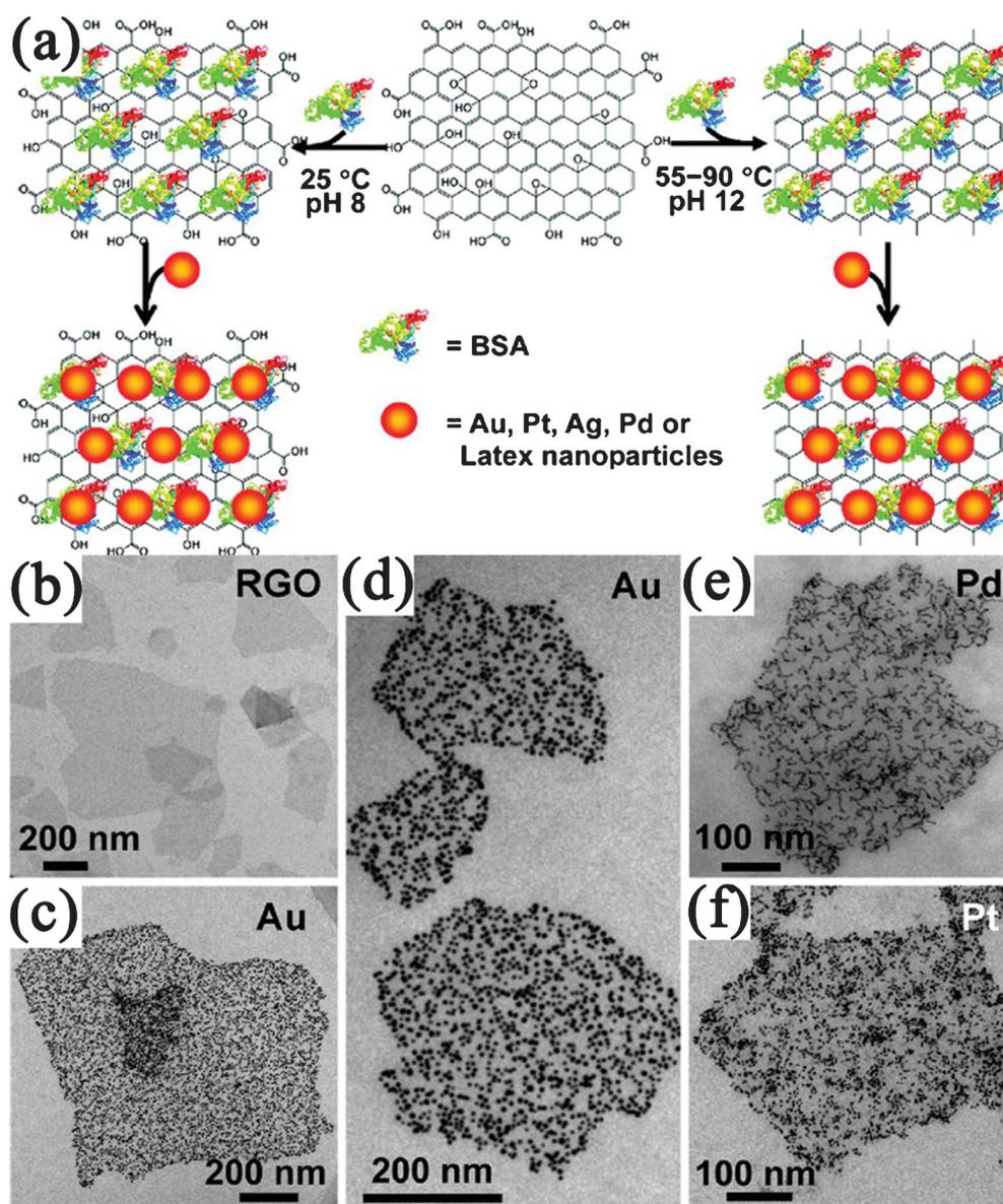
**Fig. 9** (a) Illustration of assembly of noble metal NPs on GO/RGO nanosheets with the assistance of BSA. TEM images of (b) BSA–RGO nanosheets and BSA–RGO supported (c,d) Au, (e) Pd, and (f) Pt NPs. Reprinted with permission from ref. 345. Copyright 2010, American Chemical Society.
