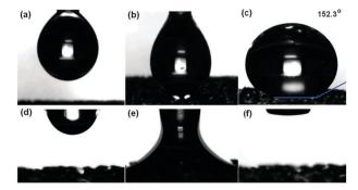
Fig. 3 Video snapshots of the wetting behaviour of a water droplet (a, b, c) and a compressor oil droplet (d, e, f) placed onto the surface of a graphene-CNT hybrid foam.
