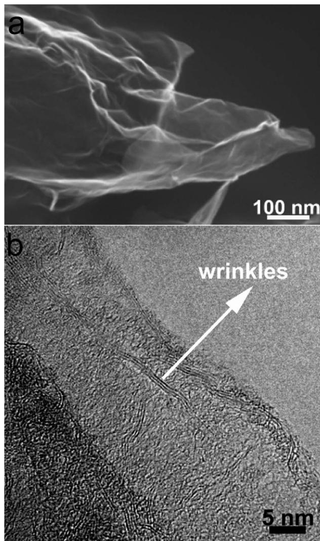
Fig. 1 (a) SEM and (b) HRTEM images of original GNSs.
