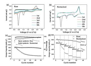
**Fig. 3** Electrochemical properties of raw and restacked MoS<sub>2</sub>: cyclic voltammograms of (a) raw and (b) restacked MoS<sub>2</sub> at a scanning rate of 0.2 mV s<sup>-1</sup>; (c) cycling performances at a current density of 50 mA g<sup>-1</sup>; (d) rate capabilities at different current densities (discharge current density was kept at 50 mA g<sup>-1</sup>).
