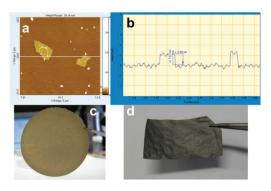
**Fig. 1** (a) and (b) AFM scan of two graphene oxide sheets, showing a single layer height of about 1 nm and about  $1 \times 1 \mu m$  wide (also determined by DLS, Fig. S3 (ESI $^{\dagger}$ )). (c) Si–graphene oxide (SGO) composite paper. (d) Si–graphene (SG) composite paper obtained by reduction of SGO.
