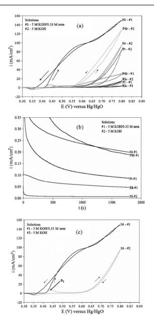
**Fig. 2** Anode catalyst analysis at 25 °C: (a) cyclic voltammograms obtained in 5 M KOH with and without the presence of urea on Ti-foil supported electrodes with a 10 mV s<sup>-1</sup> scan; (b) constant voltage test with 1.4 V potential step with 5 M KOH–0.33 M urea; (c) cyclic voltammogram of Ni/Ti electrode in the absence (grey) and presence (black) of 0.33 M KOH in 5 M KOH solution.
