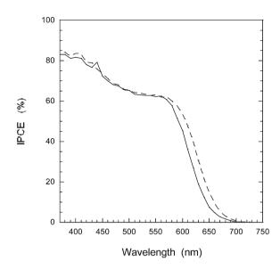
Fig. 4 IPCE spectra for dye sensitized TiO<sub>2</sub> solar cells with (---) and without scattering layer (—). The electrolyte was 0.6 M TBAI, 0.1 M LiI, 0.05 M I<sub>2</sub>, and 0.5 M 4-TBP in MeCN.
