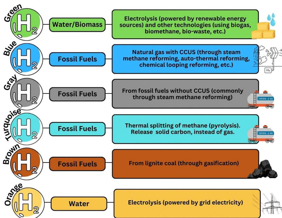
Fig. 2 Different colors of hydrogen by the technologies and feedstocks.<sup>5,30,31</sup>
