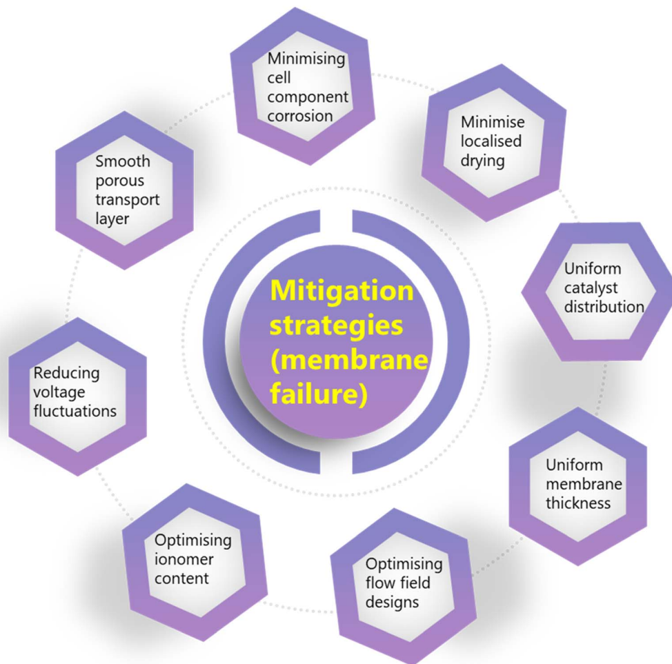
Fig. 14 An analysis chart shows some common mitigation strategies for minimizing membrane degradation in electrolyser and fuel cells.
