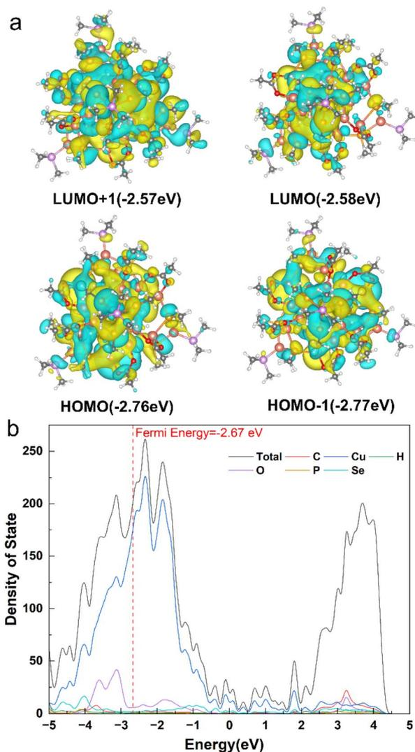
Fig. 4 (a) Frontier orbitals of  $\text{Cu}_{47}\text{H}_{12}$  cluster; (b) the total density of states and projected density of states of  $\text{Cu}_{47}\text{H}_{12}$  cluster. Color legend: Cu bronze, Se lime, P pink, O red, C gray, and H white.
