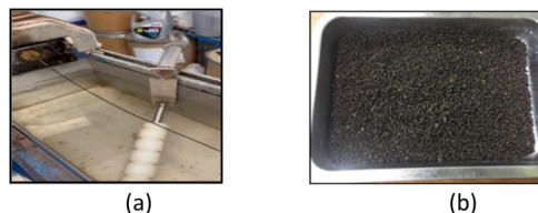
Fig. 3 Extruded bio-composite materials at different processing stages: (a) continuous strands from twin-screw extrusion; (b) pelletized granules after mechanical grinding.
