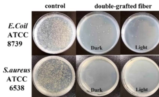
Fig. 11 Antibacterial activity of the fiber materials using colony counting method. Reprinted with permission from ref. 157. Copyright 2022, American Chemical Society.
