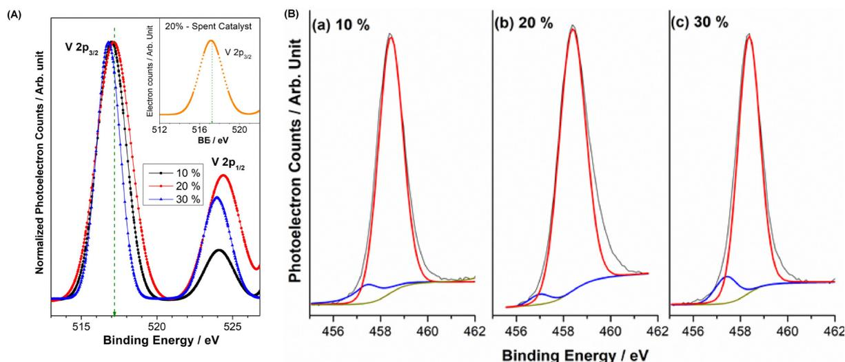
Fig. 2 (A) Vanadium 2p core level spectra recorded for different loadings of V<sub>2</sub>O<sub>5</sub> supported on TiO<sub>2</sub> and the spent catalyst. (B) Titanium 2p core level spectra recorded for different loadings of V<sub>2</sub>O<sub>5</sub> supported on TiO<sub>2</sub>.
