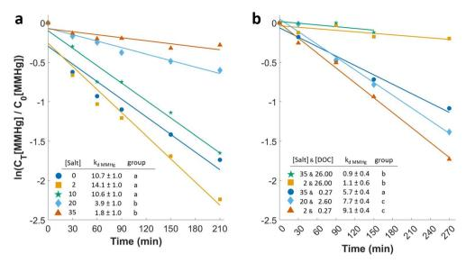
Fig. 2 Photodegradation of the added MMHg tracer over time in solutions containing (a) NaCl over a gradient from 0 to 35 g L<sup>-1</sup>. (b) Solutions containing different combinations of SRHA and NaCl concentrations. Salt concentrations are given in g L<sup>-1</sup> and DOC concentrations are stated in mg C L<sup>-1</sup>.  $k_{d \text{ MMHg}}$  refers to per day. Groups refer to *post hoc* groups based on ANOVA results (Tukey–Kramer (hsd), significance level 0.05).
