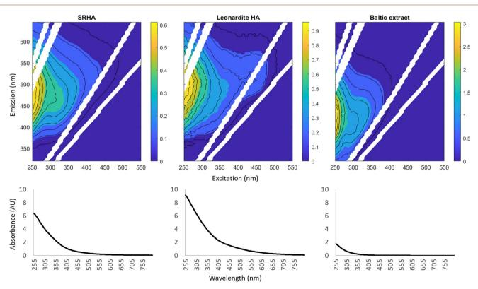
Fig. 3 Emission excitation matrices of the three different DOM extracts: SRHA, LHA, Baltic (upper panels from left to right). The color bar indicates the intensity in RAMAN Units (RU). However, note that DOC concentrations during analysis differed (SRHA: 3.53 mg C L<sup>-1</sup>; LHA: 2.8 mg C L<sup>-1</sup>; Baltic extract: 15.23 mg C L<sup>-1</sup>). Absorbance normalized as mg<sup>-1</sup> C (lower panels).
