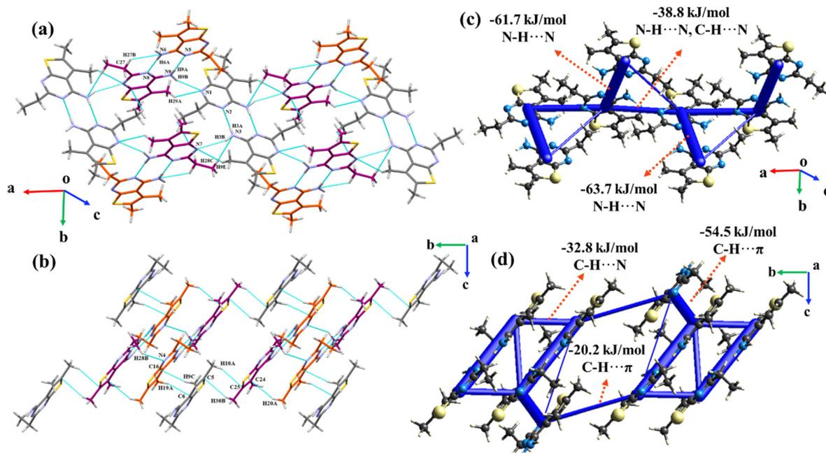
**Fig. 4** (a) Herringbone arrangement formed *via* centrosymmetric N-H...N and C-H...N interactions in compound **3**; (b) the overall packing of the molecule through C-H... $\pi$  and C-H...N interactions; (c) and (d) energy frameworks depicting the total interaction energy from the N-H...N dimer along the *ac*-plane and C-H... $\pi$ /N interactions in the *bc*-plane.
