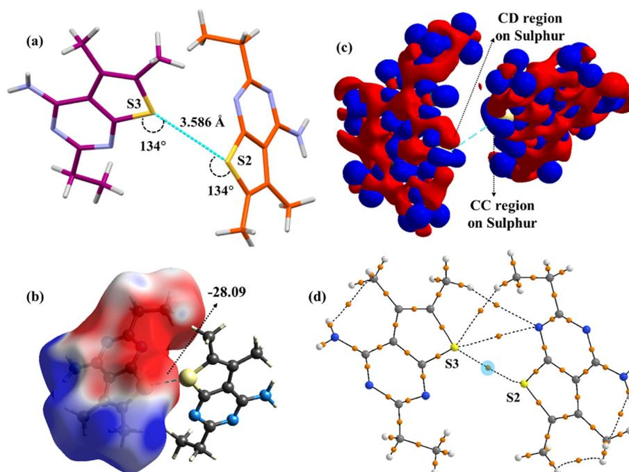
**Fig. 17** (a) Distance and directionality of S...S chalcogen interactions in compound **3**; (b) MESP mapped over the Hirshfeld surface (values in  $\text{kJ mol}^{-1}$ ); (c) deformation density plot depicting the CC and CD regions; (d) QTAIM analysis validates the existence of bond critical points (highlighted in blue circles) in dimeric motifs.
