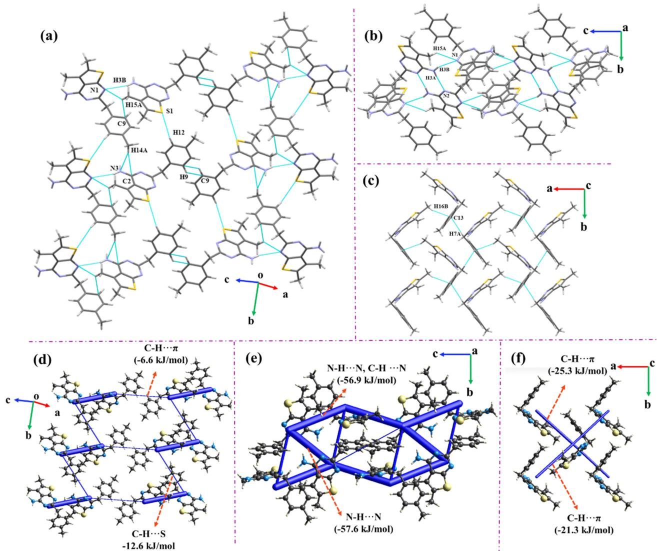
Fig. 7 (a) Crystal packing down the *b*-axis involving C-H...S/N/π interactions in compound 7; (b) herringbone pattern generated through dimeric N-H...N and C-H...N interactions in the *bc*-plane; (c) crystal packing through C-H...π along the *a*-axis; (d)–(f) energy framework diagrams depicting the total energy component.
