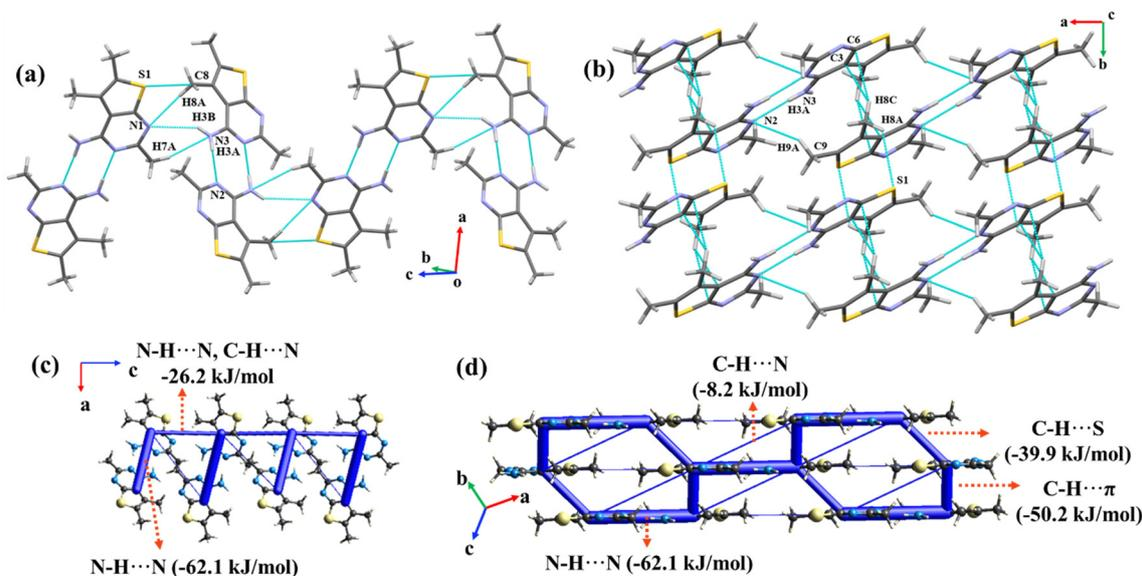
Fig. 3 (a) The packing of molecules through N–H⋯N and C–H⋯N interactions; (b) the brick layer type of stacking through N–H⋯N and C–H⋯N/S/π interactions (viewed along the  $ab$ -plane) of compound 2; (c) and (d) energy framework diagram depicting the total interaction energy values in  $\text{kJ mol}^{-1}$ .
