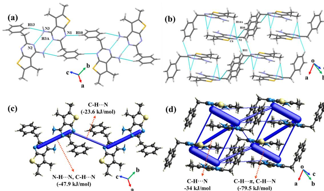
**Fig. 6** (a) The packing of the molecules *via* N-H...N and C-H...N interactions (viewed down the *ab*-plane) in compound **6**; (b) the herringbone structure generated through C-H...N and C-H... $\pi$  interactions; (c) and (d) energy framework diagrams presenting the total interaction energy component.
