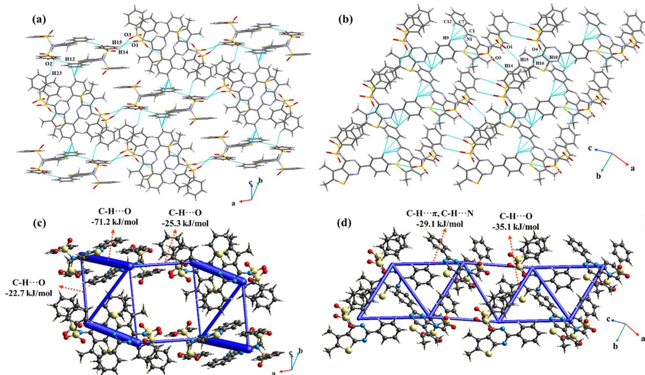
**Fig. 10** (a) Crystal packing of compound **11** through C–H...O interactions; (b) crystal packing of compound **11** through C–H...O and C9–H9... $\pi$ /N interactions; (c) and (d) energy framework diagrams representing the total interaction energy in  $\text{kJ mol}^{-1}$ .
