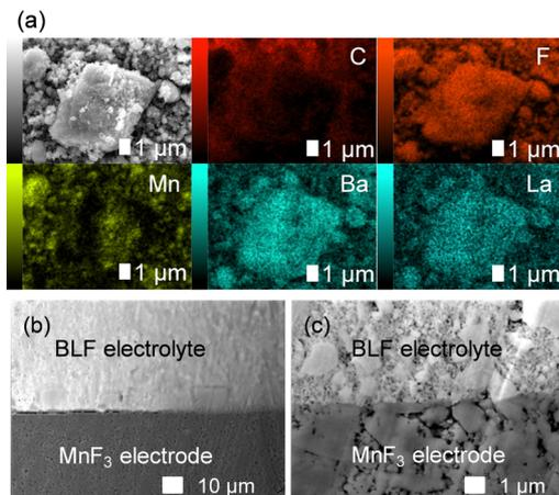
**Fig. 1** SEM images of  $\text{MnF}_3$ -based composite electrode and electrolyte/electrolyte interface for fluoride battery cell. (a) SEM image and energy dispersive spectroscopy (EDS) elemental maps of as-synthesized electrode powder. (b) and (c) Cross sectional images of BLF/ $\text{MnF}_3$  electrode interface after heating at 433 K (1000 $\times$  and 10 000 $\times$  magnification).
