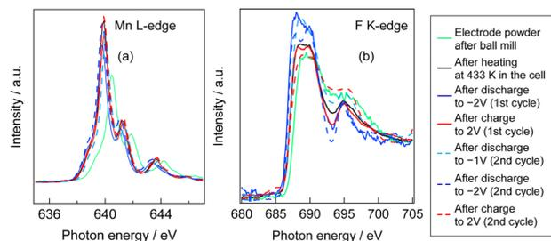
Fig. 3 (a) Mn L-edge and (b) F K-edge XAS spectra of  $\text{MnF}_3$  electrode obtained from current collector side.
