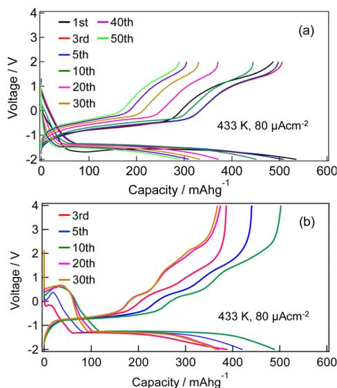
**Fig. 2** Charge-discharge profiles for all-solid-state fluoride battery with  $\text{MnF}_3$  electrode in ranges of (a)  $-2$  V to  $2$  V, and (b)  $-2$  V to  $4$  V (starting from defluorination of  $\text{MnF}_3$ ). Cell structure is  $\text{Pb}/\text{PbF}_2\text{-SnF}_2\text{-AB}/\text{BLF}/\text{MnF}_3\text{-BLF-AB}$ . The capacity was calculated based on the weight of  $\text{MnF}_3$ .
