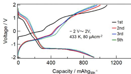
Fig. 4 Charge–discharge profiles for all-solid-state fluoride battery with metallic Mn electrode in ranges of  $-2$  V to 2 V (starting from fluorination of metallic Mn). Cell structure is  $\text{Pb}/\text{PbF}_2\text{-SnF}_2\text{-AB}/\text{BLF}/\text{Mn}\text{-BLF}\text{-AB}$ . The capacity was calculated based on the weight of Mn.
