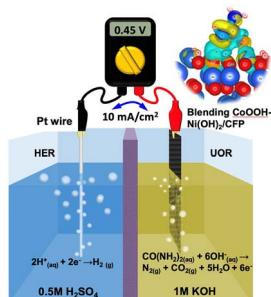
**Boosted urea electrooxidation activity by dynamic steady blending CoOOH–Ni(OH) $_2$  nanoclusters for  $\text{H}_2$  production in a pH-asymmetric electrolyzer**
