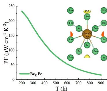
**Distinctive electronic characteristics and ultra-high thermoelectric power factor of Be–Fe intermetallics**
