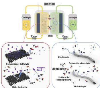
**Regulating the electrolyte network to accelerate reversible I<sup>-</sup>/I<sub>2</sub>Br<sup>-</sup> conversion and suppress zinc dendrite formation in advanced zinc–iodine flow batteries**
