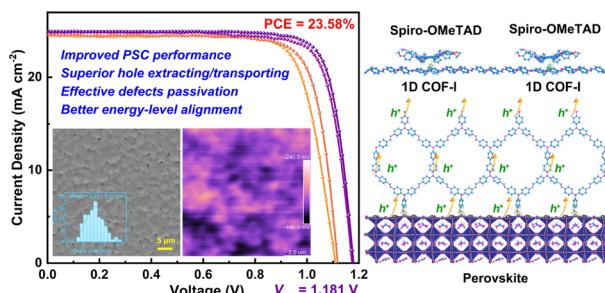
**Rational design of one-dimensional triarylamine-based covalent organic frameworks for perovskite solar cells with improved efficiency and stability**
