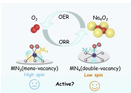
**Evolution of high spin state single-atom catalyst active centers in Na–O<sub>2</sub> batteries**
