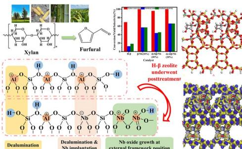
**Atomic scale niobium implantation in a dealuminated industrial H- $\beta$  zeolite catalyst for enhanced furfural production**
