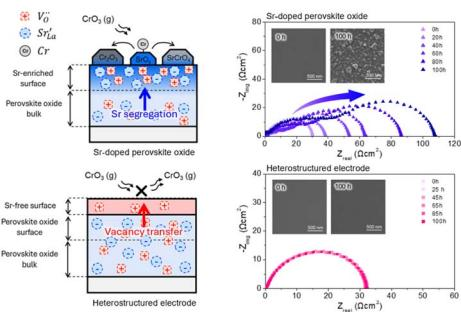
**Heterostructured electrodes for Cr-tolerant solid oxide fuel cells**
