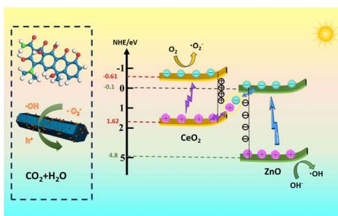
**1D rod-like {220}-faceted CeO<sub>2</sub>/ZnO S-scheme heterojunctions: design, photocatalytic mechanism and DFT calculations**
