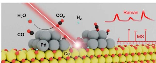
**Understanding water-gas shift reaction mechanisms at palladium–ceria interfaces using *in situ* SERS coupled with online mass spectrometry**
