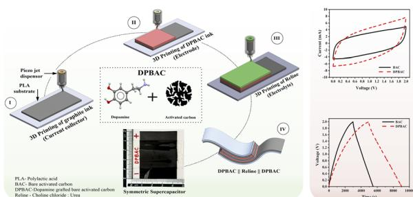
**A 3D-printed fully biocompatible supercapacitor**
