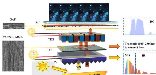
**Collecting bidirectional flow energy through a photovoltaic thermoelectric radiative cooling hybrid system to maximize the utilization of electricity from the sun and outer space**
