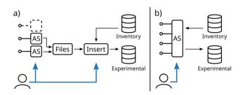
Fig. 3 Schematic communication between database and acquisition software (AS) controlling different measurement devices. Blue arrows indicate required user interaction. (a) Communication *via* exported data files (b) integrated database communication.
