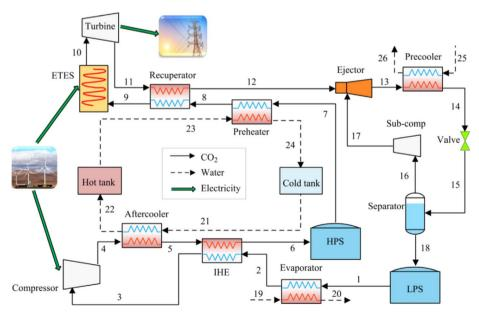
Fig. 2 A schematic of the carbon dioxide electrothermal energy storage system's cycle.<sup>43</sup>
