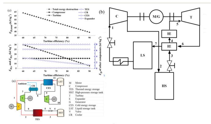
Fig. 4 (a) Compressed  $CO_2$  energy storage system based on Brayton cycle;<sup>59</sup> (b) integrated energy storage system of supercritical (transcritical)  $CO_2$  Rankine cycle and voltage shrinking refrigeration cycle;<sup>60</sup> (c) effect of turbine efficiency on exergy.<sup>59</sup>
