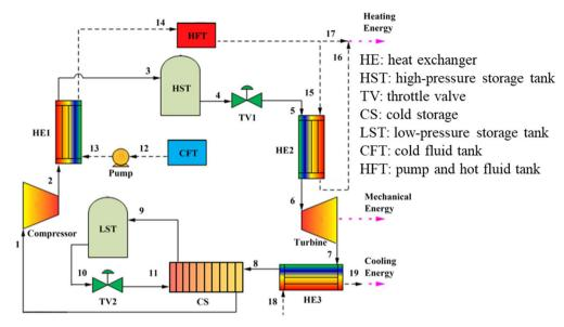
Fig. 3 Schematic diagram of CCES system. 46
