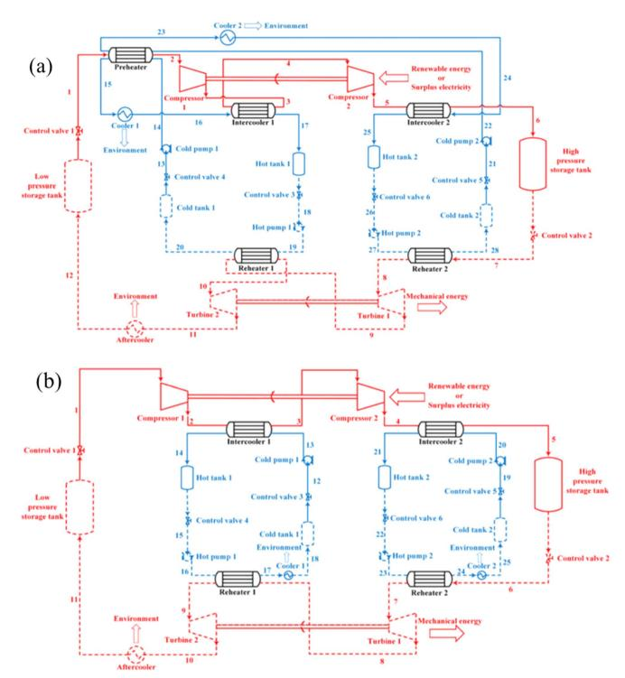
Fig. 8 (a) A cross-carbon dioxide energy storage system based on Brayton cycle;<sup>59</sup> (b) an ultra-carbon dioxide energy storage system based on Brayton cycle.<sup>59</sup>
