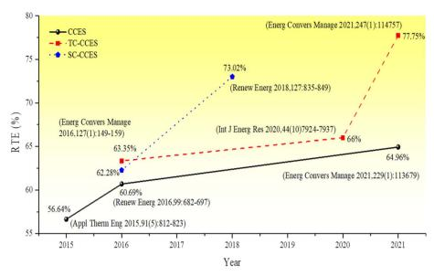
Fig. 1 Development diagram of round-trip efficiency of CCES system.
