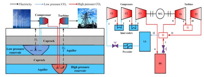
Fig. 7 A carbon dioxide energy storage system with underground rock strata.<sup>47</sup>
