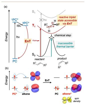
Fig. 1 (a) Overview of EnT photocatlytic processes applied to the isomerization of alkenes. (b) Schematic frontier molecular orbital diagram illustrating the sensitization of alkenes *via* EnT. Molecular orbitals of ethene and spin density for its triplet state are represented on B3LYP-optimized geometries with isovalues of 0.02 and 0.06, respectively.
