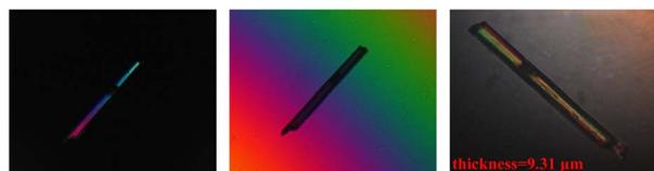
Fig. 5 Experimental birefringence at 546 nm for  $\text{Pb}_2(\text{SeO}_3)(\text{SiF}_6)$ .
