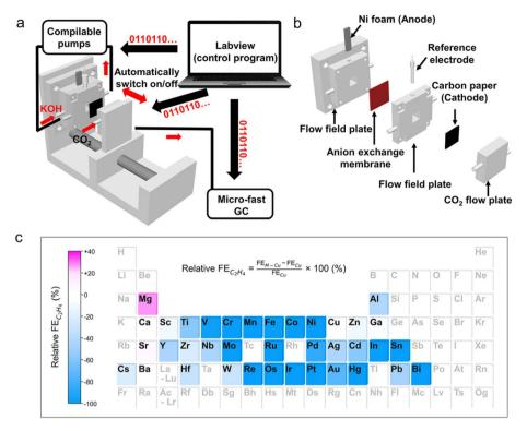
Fig. 9 Fast screening platform for screening bimetallic catalysts for the CO<sub>2</sub>RR. (a) Schematic illustration of the fast screening platform for the  $CO_2RR$ . (b) Exploded view of a 3D-printed flow cell. (c) Heat map of the relative FE of  $C_2H_4$  over Cu-based bimetallic catalysts. Elements in black font represent tested metal salt additives and elements in grey font represent the untested ones. Reproduced with permission from ref. 106 Copyright 2022, Wiley.
