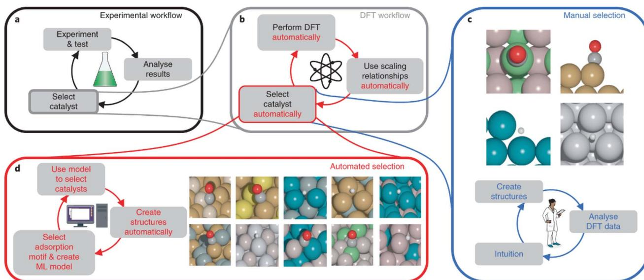
Fig. 15 Workflow for automating theoretical materials discovery. (a) and (b) The experimental workflow for catalyst discovery is accelerated by the *ab initio* DFT workflow. (c) Scientists relied on their expertise and experimental results to screen data for DFT calculations traditionally. (d) This work uses ML to select DFT data automatically and systematically. Reproduced with permission from ref. 31 Copyright 2018, Springer Nature.
