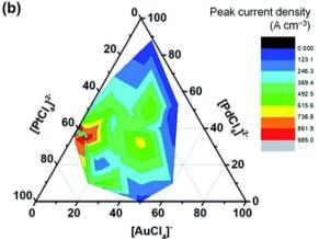
Fig. 12 Bayesian optimization of the methanol electro-oxidation process. (a) Peak current density of methanol electro-oxidation as a function of the number of BO rounds. (b) A contour plot showing the peak current density and a ternary plot depicting the chemical composition in the electrolyte solution. Reproduced with permission from ref. 20 Copyright 2020, Royal Chemical Society.
