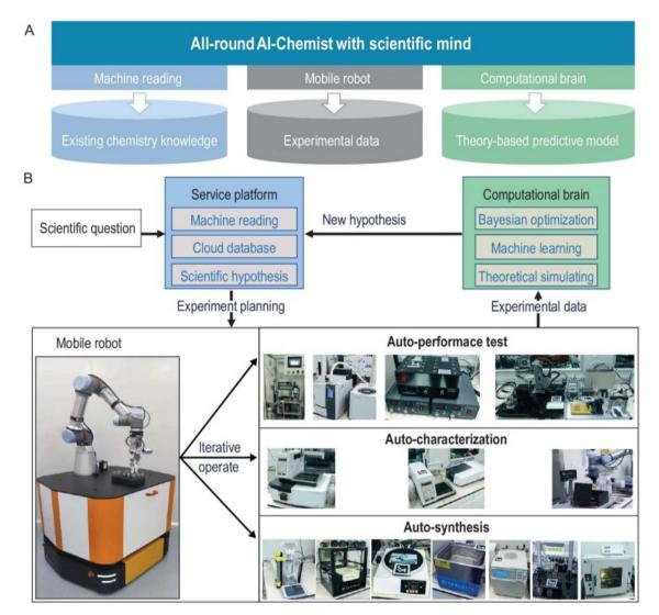
Fig. 7 Design of the all-round Al-Chemist with a scientific mind. It includes three modules for chemistry knowledge, autonomous experimentation, and theoretical computation and machine learning (A). The workflow of the Al-Chemist to study various systems are shown in (B). Reproduced with permission from ref. 5 Copyright 2022, China Science Publishing & Media Ltd.
