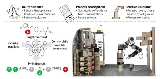
Fig. 11 A robotically reconfigurable flow chemistry platform. Reproduced with permission from ref. 123 Copyright 2019, AAAS.
