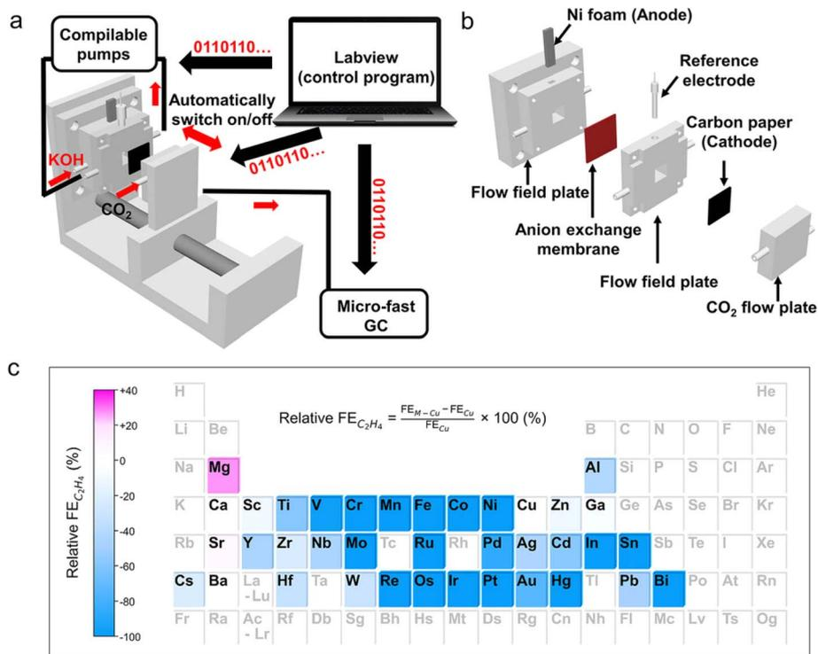
Fig. 9 Fast screening platform for screening bimetallic catalysts for the CO<sub>2</sub>RR. (a) Schematic illustration of the fast screening platform for the CO<sub>2</sub>RR. (b) Exploded view of a 3D-printed flow cell. (c) Heat map of the relative FE of C<sub>2</sub>H<sub>4</sub> over Cu-based bimetallic catalysts. Elements in black font represent tested metal salt additives and elements in grey font represent the untested ones. Reproduced with permission from ref. 106 Copyright 2022, Wiley.
