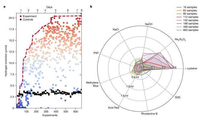
Fig. 13 (a) Maximum rate of hydrogen evolution from photolyzed water reaching 21.05  $\mu$ mol h<sup>-1</sup> after 688 experiments during an 8-day autonomous search. (b) Radar plot illustrating the sampling in the search space during experimentation. Reproduced with permission from ref. 4 Copyright 2020, Springer Nature.
