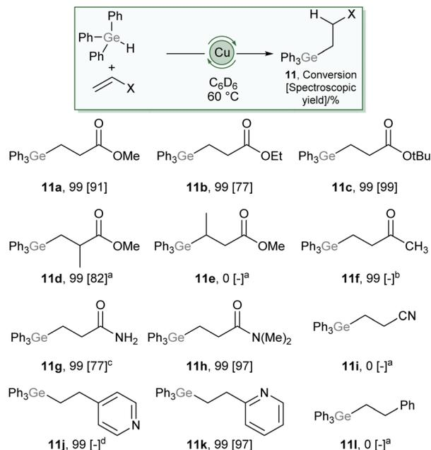
Scheme 6 Scope of the hydrogermylation of Michael-acceptors catalysed by 10 mol%  $(\text{SIMes})\text{CuOtBu}$ . For full details see ESI,<sup>†</sup> values in brackets are spectroscopic yields relative to an internal standard. (a) 100 °C, (b) 80 °C, provided an intractable mixture with no evidence of desired product, (c) reaction performed in  $d_8$ -THF at 100 °C, (d) provided an intractable mixture including desired product.
