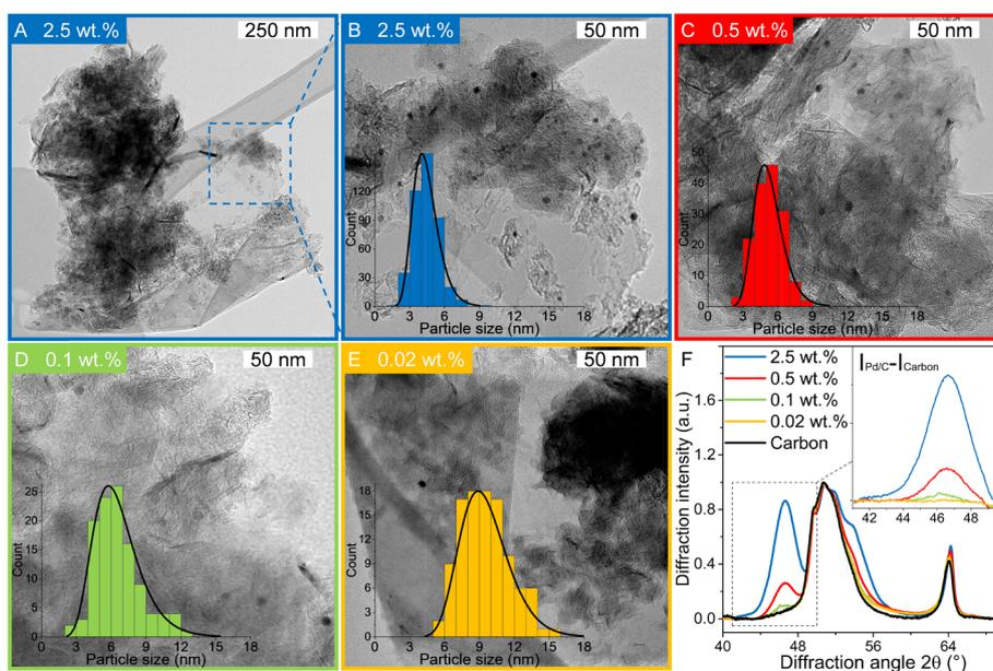
**Fig. 2** Catalyst characterisation. (A–E) Transmission Electron Microscopy (TEM) images of Pd/C catalysts with Pd weight loading of (A) 2.5 wt% and high (B) magnification, (C) 0.5 wt% (D) 0.1 wt% and (E) 0.02 wt%. Insets shown size histograms of the individually measured diameters from TEM and lognormal fit to the distribution. (F) X-ray diffractogram of the Pd/C catalysts. The inset shows the carbon-subtracted intensity, highlighting the Pd(111) diffraction at 46.6° 2θ.
