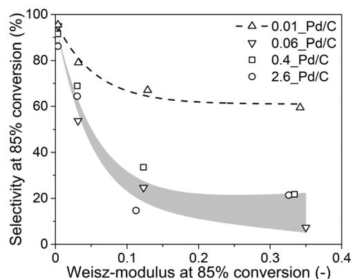
**Fig. 7** Weisz-modulus as selectivity descriptor. Comparison of the experimentally measured selectivity (taken at 85% conversion) and the calculated Weisz-modulus of the tested catalysts. Lines as a guide for the eye.
