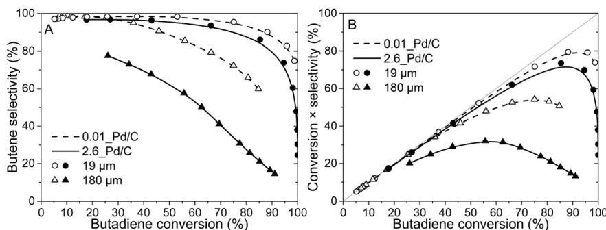
Fig. 4 Grain size affects the butene selectivity. (A) Selectivity as function of butadiene conversion of 2.6\_Pd/C (solid line, filled symbols) and 0.01\_Pd/C (dashed line, open symbols) catalysts with an average grain size of 19  $\mu\text{m}$  (circles) or 180  $\mu\text{m}$  (triangles). (B) Butenes yield during the selective hydrogenation of butadiene.
