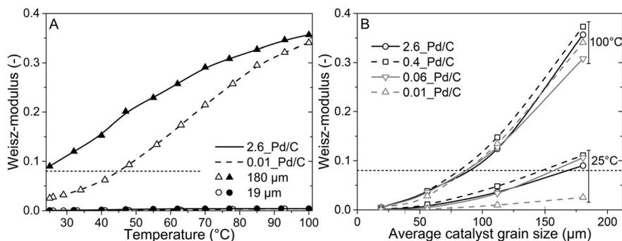
Fig. 5 Larger grains induce internal diffusion limitations. (A) Weisz-modulus of 2.6\_Pd/C (solid line, filled symbols) and 0.01\_Pd/C (dashed line, open symbols) catalysts with average catalyst grain size of 19  $\mu\text{m}$  (circles) or 180  $\mu\text{m}$  (triangles). (B) Overview of the Weisz-moduli for the tested combinations of Pd loading and grain size at lowest (25  $^{\circ}\text{C}$ ) and highest (100  $^{\circ}\text{C}$ ) tested temperature.
