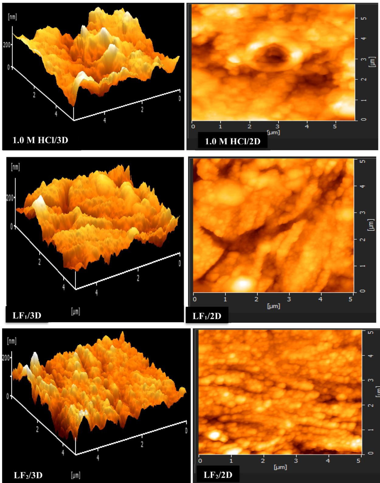
Fig. 6 AFM images (2D and 3D) were captured for C.S specimens both in the non-existent and in the existence of  $1 \times 10^{-3}$  M concentrations of LF<sub>1</sub> & LF<sub>2</sub>.
