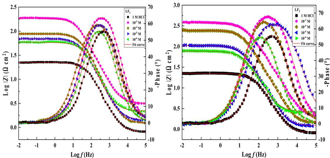
Fig. 3 Bode plots & phase angle spectral representations of Bode for the impedance spectroscopy system in a 1.0 M HCl solution, both with and without different  $LF_1$  &  $LF_2$  concentrations at 303 K.
