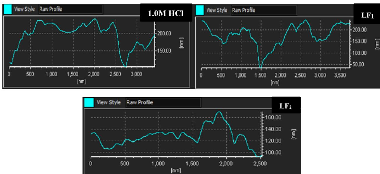
Fig. 7 Displays the relative-height profiles extracted from 3D/2D AFM images at a temperature of 303 K.
