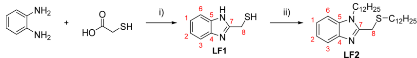
Scheme 1 General procedure for the synthesis of LF 1 and LF 2 . Reagents and conditions: (i) 4 N-HCl, 2 h, reflux; (ii) C 12 H 25 Br, K 2 CO 3 , TBAB, DMF, RT.
