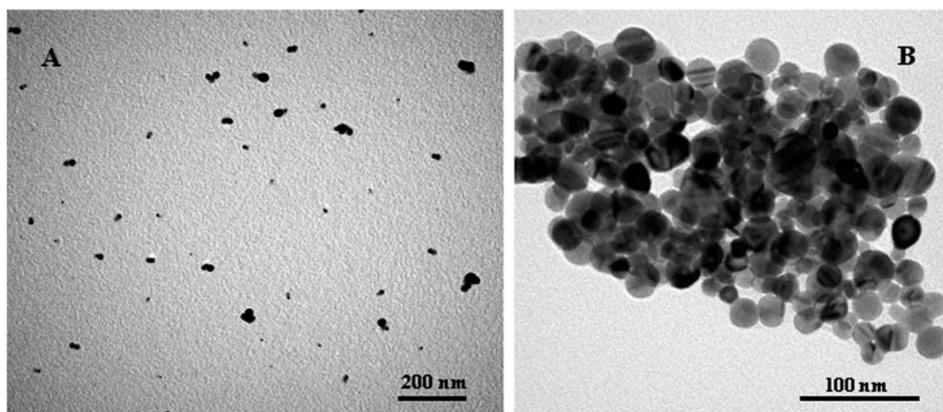
Fig. 12 TEM images of the AgNPs solution (0.075 nM) mixed with 300 nM MSO in the (A) absence or (B) presence of 500 nM  $\text{Hg}^{2+}$  after the addition of 60 mM NaCl. Reproduced with permission from ref. 115, copyright 2024, ACS Appl. Mater. Interfaces.
