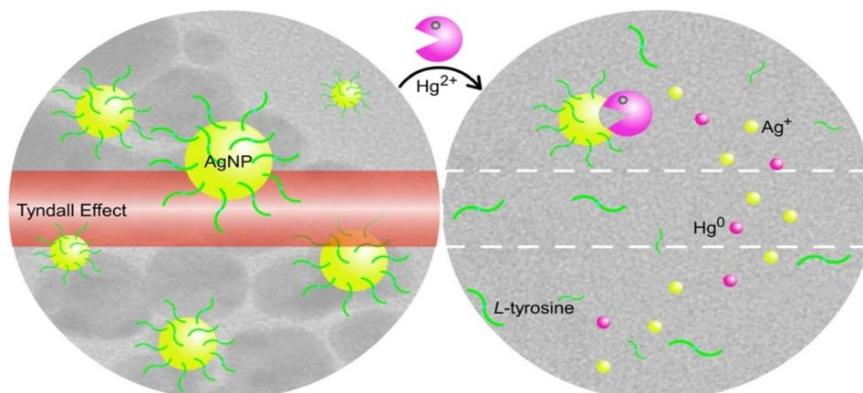
Fig. 11 Sensing of mercury with tyrosine-stabilized AgNPs involving the Tyndall effect. Reproduced with permission from ref. 117, copyright 2024, *Sens. Actuators B: Chem.*
