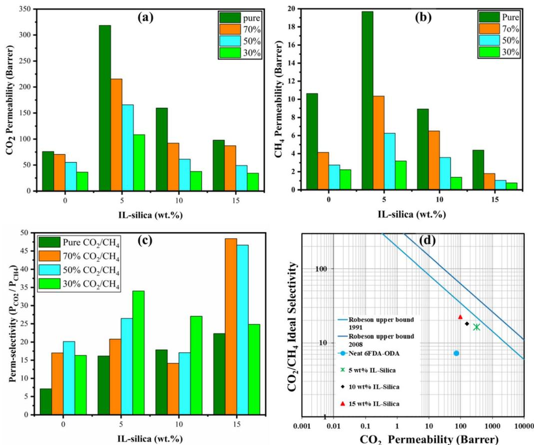
Fig. 11 Transport properties under different gas composition in a membrane with varying filler loadings (a) CO<sub>2</sub> gas permeability, (b) CH<sub>4</sub> gas permeability, (c) CO<sub>2</sub>/CH<sub>4</sub> permeability–selectivity; (d) membrane performance as compared with Robeson upper bounds.
