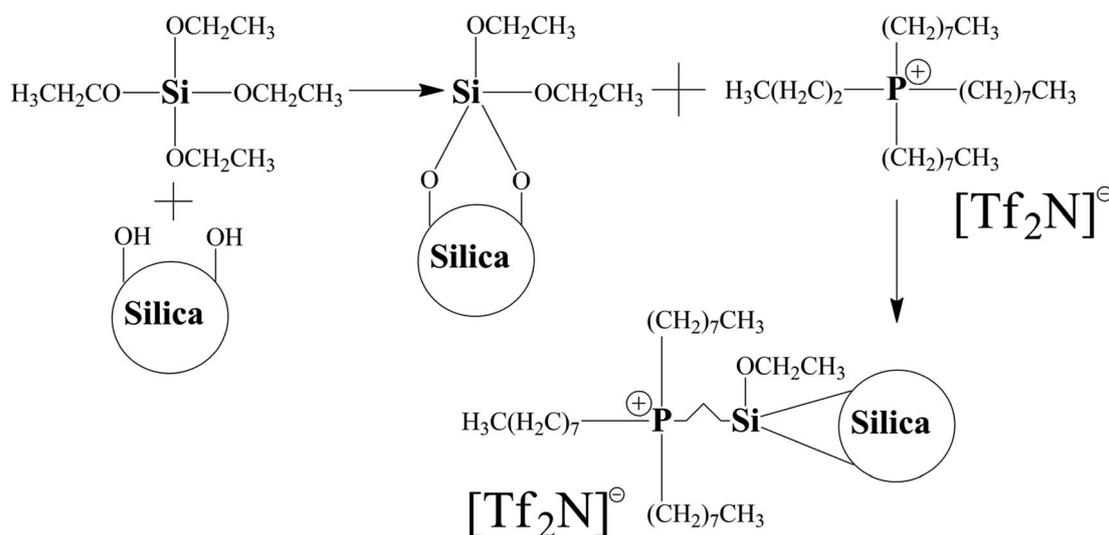
Fig. 2 Procedure to support IL on silica surface.
