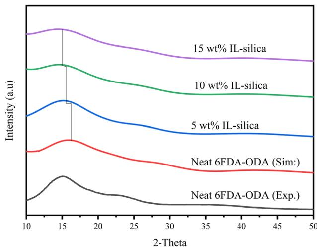
Fig. 8 X-ray scattering patterns for 6FDA-ODA polymer with different weight percentages of IL-silica (experimental XRD data for neat 6FDA-ODA is extracted from the graph<sup>89</sup>).
