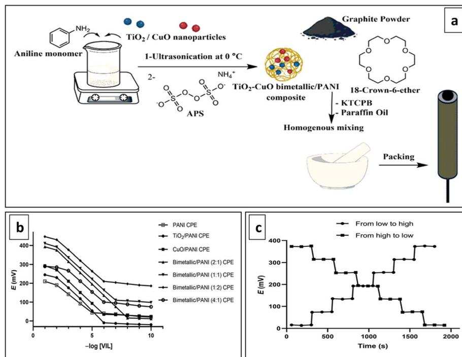
Fig. 10 (a) Diagram outlining the fabrication process of the electrode with  $\text{TiO}_2\text{-CuO}$  bimetallic/PANI nanocomposite transducer, (b) potentiometric responses and (c) dynamic response time of the electrode. Reproduced with permission.<sup>149</sup> Copyright 2023, MDPI, Basel, Switzerland.
