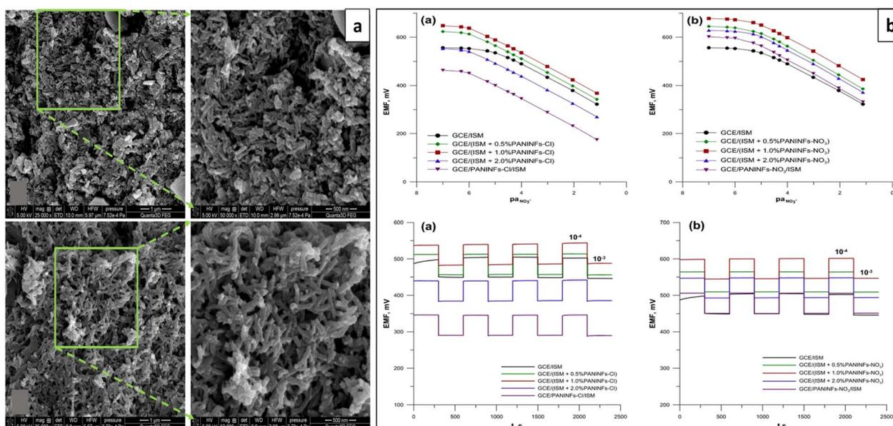
Fig. 6 (a) SEM micrographs of PANI NFs-Cl (upper) and PANI NFs-NO<sub>3</sub> (lower) and (b) ISE performances. Reproduced with permission.<sup>53</sup> Copyright 2021, Springer.
