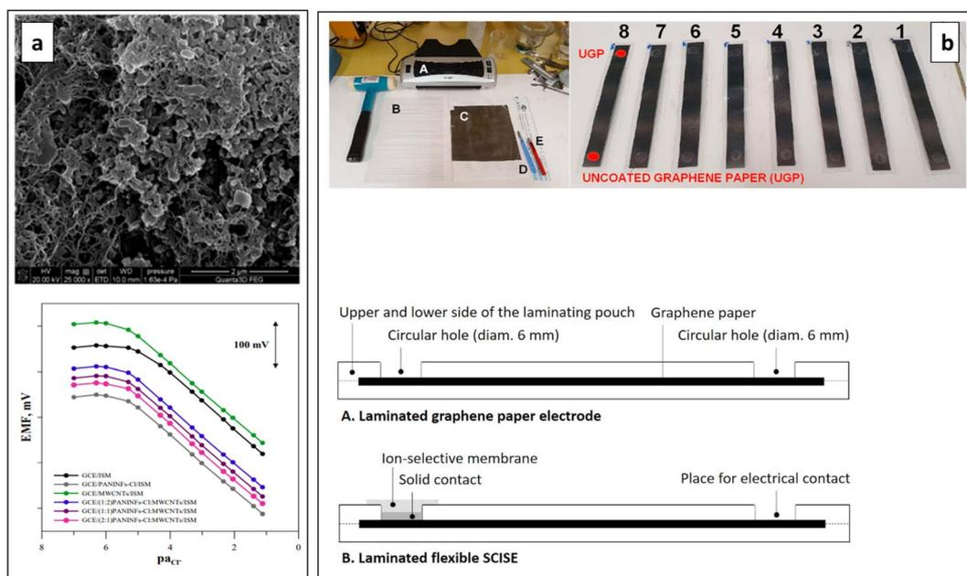
Fig. 9 (a) SEM image of PANI NFs-Cl:MWCNTs composite (upper) and potentiometric responses of the SC-ISEs (lower). Reproduced with permission.<sup>76</sup> Copyright 2022, MDPI, Basel, Switzerland. (b) Required equipment for the fabrication process, laminated graphene paper electrodes (upper) and schematic side view of the flexible SC-ISEs (lower). Reproduced with permission.<sup>146</sup> Copyright 2021, Elsevier.
