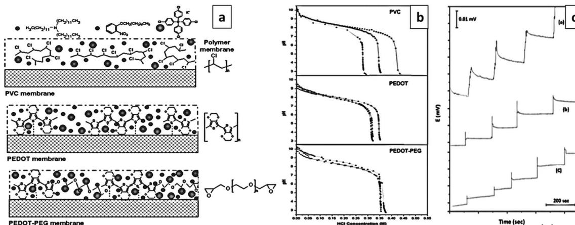
Fig. 15 (a) Diagram outlining the ISMs (PVC, PEDOT and PEDOT-PEG), (b) repetition of the response and (c) comparison of kinetic responses. Reproduced with permission.<sup>177</sup> Copyright 2014, MDPI, Basel, Switzerland.
