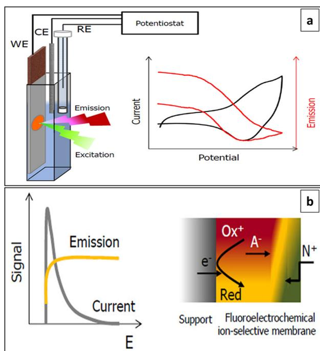
Fig. 16 (a) *In situ* transduction of electrochemical responses to emission change signal of ISEs operating under non-zero-current conditions. (b) Schematic representation of the mechanism of fluoro-electrochemical ISMs. Reproduced with permission.<sup>175</sup> Copyright 2021, American Chemical Society.
