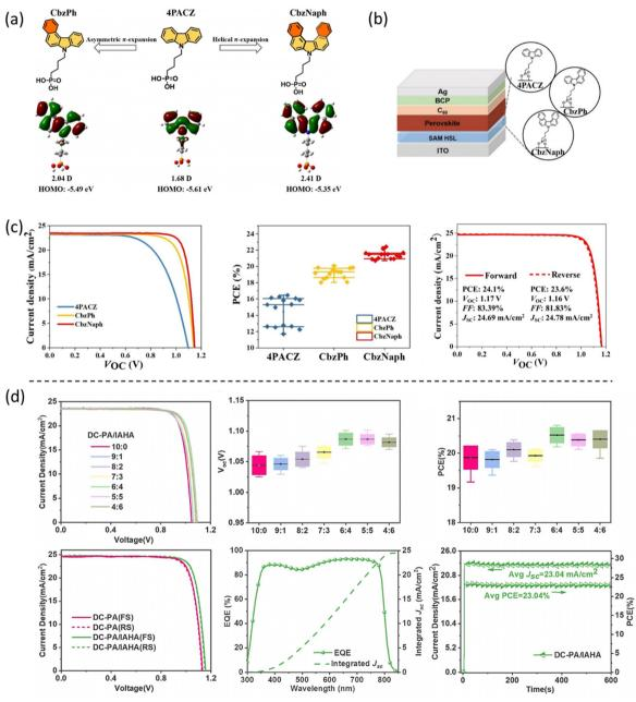
Fig. 7 (a) The π-expanded carbazole-based molecules and their calculated molecular dipole. (b) Device architecture of the CbzPh and CbzNaph-based p-i-n PSC and (c) their corresponding device performance. Reproduced with permission.<sup>27</sup> Copyright 2022, Wiley. (d) Device performance is based on the co-assembled DC-PA and IAHA monolayer substrates. Reproduced with permission.<sup>38</sup> Copyright 2022, Wiley.
