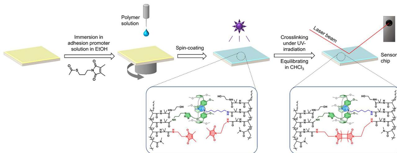
**Fig. 7** SPR sample preparation. Gold-coated N-LaSF9 wafer is immersed in an adhesion promoter solution overnight. Then, a polymer (mixture) solution is spin-coated onto the wafer, followed by drying *in vacuo* and crosslinking by UV-irradiation. After equilibrating in  $\text{CHCl}_3$  overnight the sensor chip can be measured.
