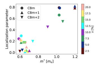
Fig. 8 Localization parameter L mapped against the effective mass  $m^*$  for the 3 lowest states in the conduction band at  $\Gamma$ . States with  $m^* < 0.8 m_{\rm e}$  are densely clustered in the area with low L, while the ones with higher effective mass are more dispersed, but still clearly correspond to higher values of L.
