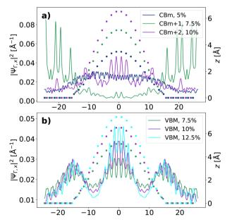
Fig. 7 Normalized wave-function distribution averaged in the (y, z)-plane of the (a) CBm and (b) VBM at  $\Gamma$  calculated for selected nanowrinkles with s=7.5%, s=10%, and s=12.5%. The z-coordinates of the Mo atoms in the nanowrinkles are shown for reference by colored dots.
