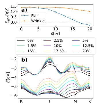
Fig. 4 (a) Band gap ( $E_{gap}$ ) vs. strain (s) of the considered MoSe<sub>2</sub> nanowrinkles (orange) and of the flat monolayers under the same amount of uniaxial strain in their hexagonal UC (blue). (b) Highest-occupied and lowest-unoccupied band of flat MoSe<sub>2</sub> under the displayed values of strain. The deformation of the BZ leads to different distances between the high-symmetry points in the K-path and hence they are shown separately for each strain value.
