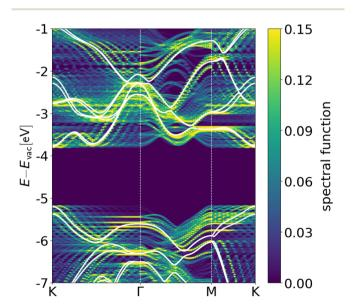
Fig. 3 Unfolded band structure of the nanowrinkle with s=10% represented by the spectral function. The white lines indicate the band structure of the flat and unstrained MoSe<sub>2</sub> monolayer. The energy scale is offset with respect to the vacuum level ( $E_{vac}$ ) set to zero.
