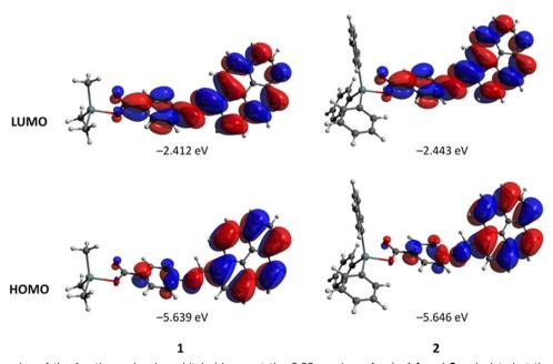
Fig. 8 Plots and energies of the frontier molecular orbitals (shown at the 0.02 a.u. isosurface) of 1 and 2, calculated at the B3LYP/ZORA-def2-TZVP(SARC-ZORA-TZVP) level and based on atom coordinates optimized at the same level. Colour scheme: Sn, light grey; O, red; N, blue; C, grey; H, white.
