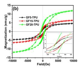
Fig. 5 Magnetic hysteresis (M-H) curve of (a) the synthesized CoFe<sub>2</sub>O<sub>4</sub> nanoparticles and (b) the developed GF-TPU nanocomposites.
