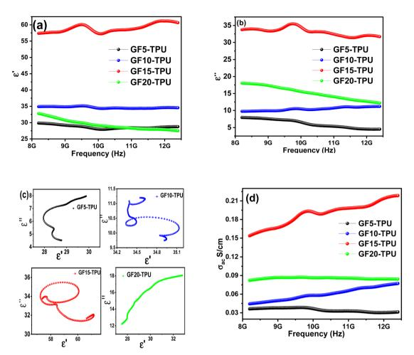
Fig. 9 (a) The real part of the permittivity  $\varepsilon'$ , (b) imaginary part of permittivity  $\varepsilon''$  as a function of the frequency, (c) Cole–Cole plot, and (d) a.c. conductivity  $\sigma_{ac}$  as a function of frequency for all the developed GF–TPU nanocomposites.
