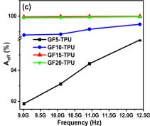
Fig. 7 (a) The comparison plot of the contribution of  $SE_{A}$ ,  $SE_{R}$  and  $SE_{T}$  for the developed GF–TPU nanocomposites, (b) power coefficients for the GF15–TPU nanocomposite, and (c)  $A_{eff}$  of the developed GF–TPU nanocomposites as a function of frequency.
