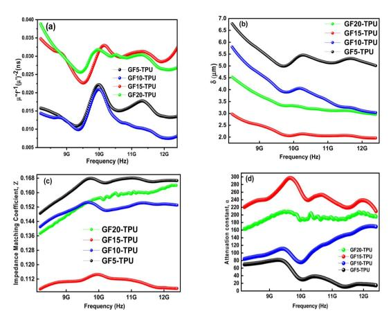
Fig. 11 Variation of (a) eddy current loss,  $C_0$ , (b) skin-depth,  $\delta$ , (c) impedance matching coefficient, Z, and (d) attenuation constant,  $\alpha$ , as a function of the frequency for all the developed GF-TPU nanocomposites.
