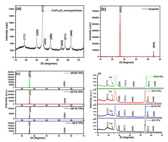
Fig. 2 XRD pattern of (a)  $CoFe_2O_4$  nanoparticles, (b) graphite, (c) all the developed GF-TPU nanocomposites; and (d) magnified XRD pattern of all the developed GF-TPU nanocomposites.
