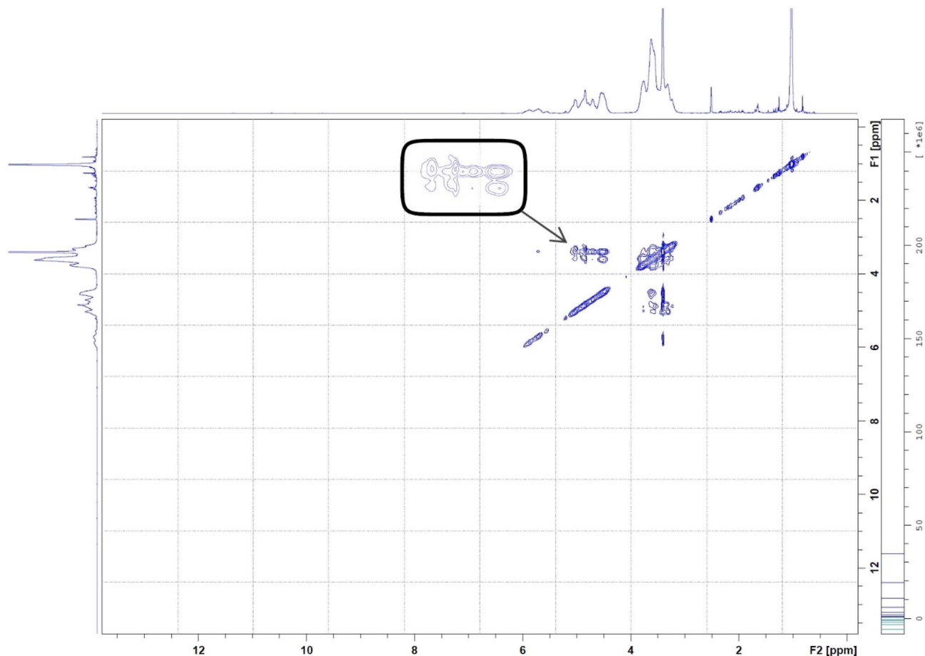
Fig. 5 2D HNMR (NOESY) spectrum of BO-ICs. The spectrum showed the interaction between BO and HP \beta CD's protons.
