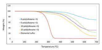
Fig. 8 Comparative TGA thermograms of X-poly(siloxane-r-S) (X = wt%S); X = 0 (blue), 5 (purple), 10 (green), 15 (yellow), and  $S_8$  (red).
