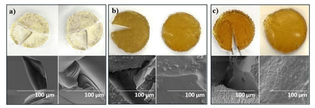
Fig. 10 Thermally repairable properties of polysiloxane samples with varying wt% S (X) and their corresponding SEM images, shown before (left) and after (right) the healing process for X-poly(siloxane-r-S); X = (a) 0 (b) 5 (c) 10.
