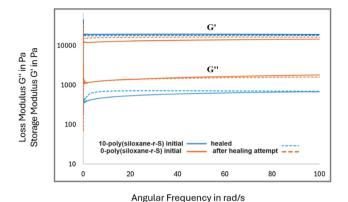
Fig. 11 Storage modulus (G') and loss modulus (G'') measurements of 0poly(siloxane-r-S) (orange) and 0-poly(siloxane-r-S) (blue) initial (solid line) and after healing attempt (dotted line).
