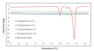
Fig. 9 Comparative DSC thermograms of X-poly(siloxane-r-S) (X = wt% S); X = 0 (blue), 5 (purple), 10 (green), and 15 (yellow) and S<sub>8</sub> (red).
