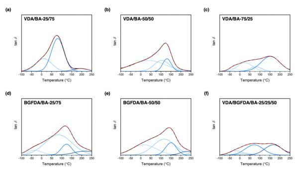
Fig. 2 Deconvolution of  $\tan \delta$  curves of acrylate networks. The red dashed line (---) denotes the original curve, and the black solid line (-) is the integrated result of deconvoluted curves. All y-axes are on the same scale.
