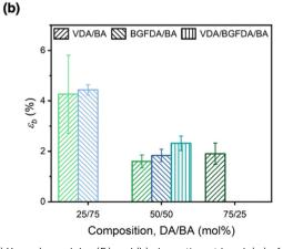
Fig. 4 (a) Young's modulus ( $E_t$ ) and (b) elongation at break ( $\varepsilon_b$ ) of acrylate networks. Error bars represent the standard deviations from triplicate measurements
