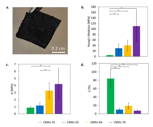
Fig. 4 Mechanical properties of CMXn thin films. Tensile test measurements for dried CMXn films: (a) close-up image of CMXn-55 film with dimensions of 0.5 mm  $\times$  0.5 mm, (b) Young's modulus and ultimate (c) stress ( $\sigma$ )  $\delta$  (d) strain ( $\epsilon$ ). A t-test was applied to determine if the samples were statistically different if lower than p = 0.05
