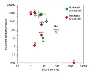
Fig. 6 Comparison of maximum ultimate strain (ε) and maximum conductivity achieved by other MXene composite films using different manufacturing techniques. Nomenclature and numerical values are shown in Table S1 (ESI†). Further mechanical properties and assembly techniques are shown in Table S2 (ESI†)
